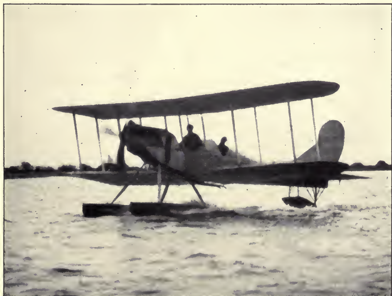
HYDRO-AEROPLANE H.R.E.3. R.A.F. Design for the "Naval Wing" (Now R.N. Air Service) in 1912.
