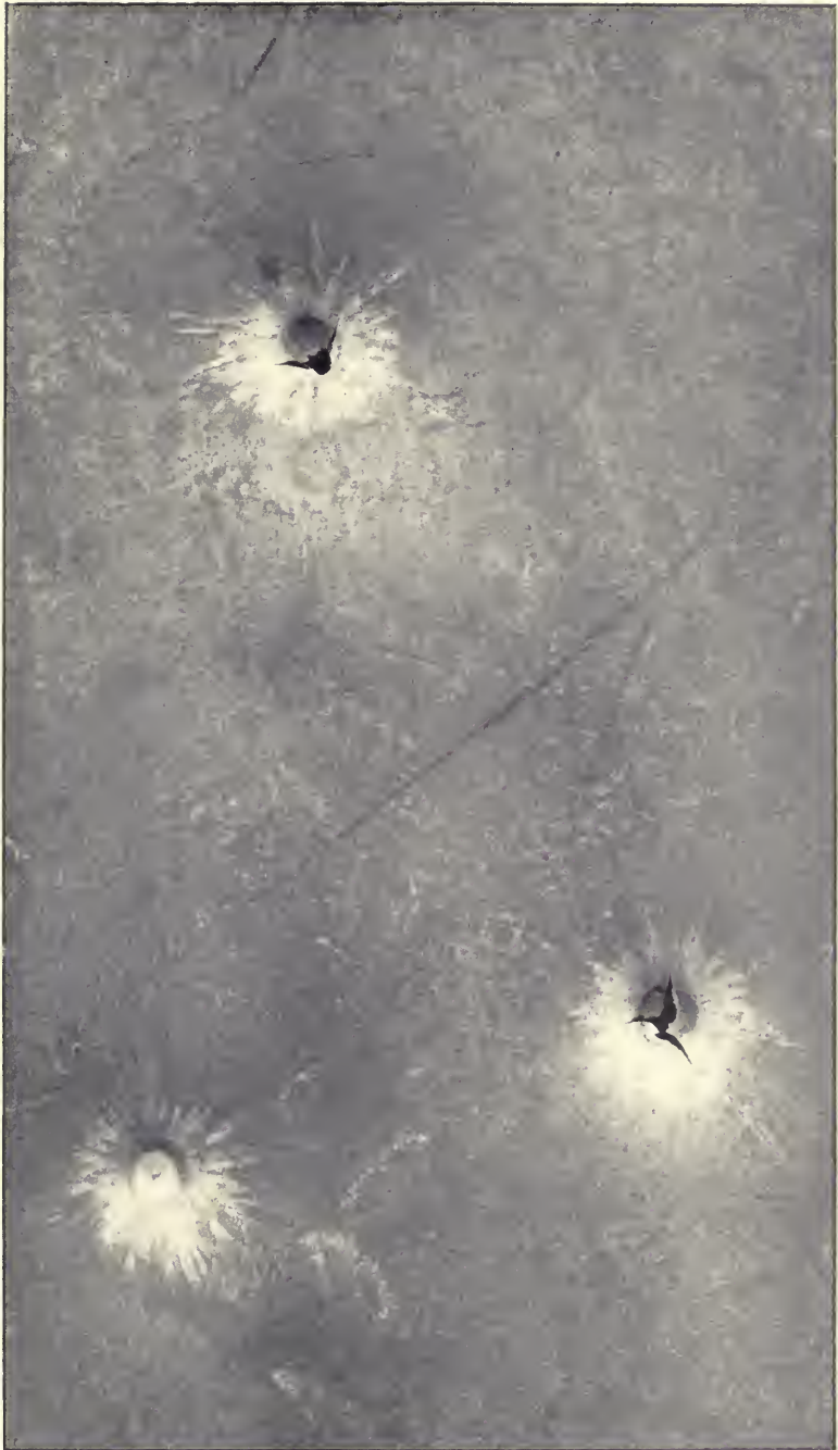
TEST OF "BULLET-PROOF" STEEL PLATE, 3 M.M. THICK. Range 300 yards. Service Rifle. Mark VI. Ammunition.
