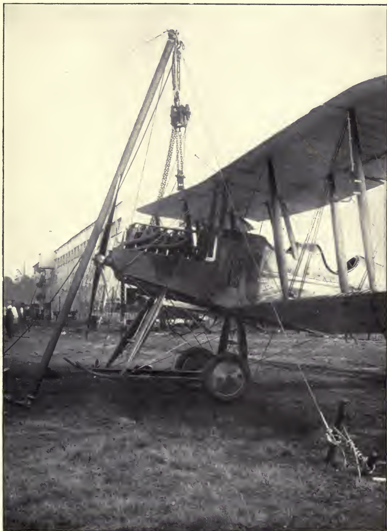
R.A.F. TYPE R.E.5. An "R.E. Portable" Tent Pole is shown used as Derrick for dismounting Engine
